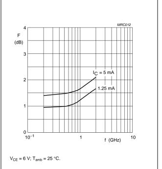
Fig.11 Minimum noise figure as a function of frequency.
