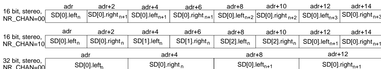
Figure 2: Examples of Audio Out Memory DMA Formats
