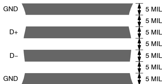
Figure 23. Typical Arrangement of Signal Tracks
