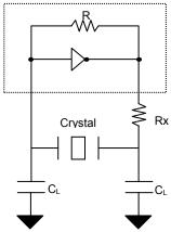
$$\begin{split} C_L &= 2^*(C_P - C_S),\\ \text{Where } C_P &= \text{Load capacitance of crystal}\\ C_S &= \text{Stray capacitance due to } C_{\text{IN}}, \text{PCB}, \text{Trace etc.} \end{split}$$
