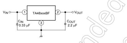
• Be sure to connect a capacitor near the input terminal and output terminal between both terminals and GND. The use of a monolithic ceramic capacitor (B Characteristic or X7R) of low ESR (equivalent series resistance) is recommended. The IC may oscillate due to external conditions (output current, temperature, or the type of the capacitor used). The type of capacitor required must be determined by the actual application circuit in which the IC is used.
