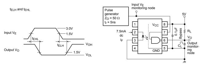
(\*) CL is approximately 15pF which includes probe and stray wiring capacitance.
