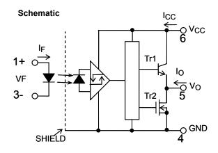
$0.1~\mu F$  bypass capacitor must be connected between pins 6 and 4.
