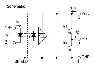
0.1 µF bypass capacitor must be connected between pins 6 and 4. Unit in mm
