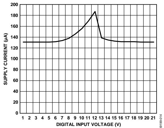
Figure 15. AD5512A/AD5542A Supply Current vs. Digital Input Voltage
