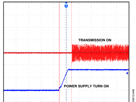
Figure 17. Time to Initialize, Including Reset, 40\text{ ms}/\text{DIV}
