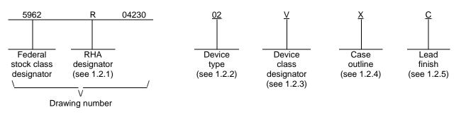
1.2.1 <u>RHA designator</u>. Device classes Q and V RHA marked devices meet the MIL-PRF-38535 specified RHA levels and are marked with the appropriate RHA designator. A dash (-) indicates a non-RHA device.
