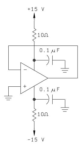
FIGURE 2. Radiation exposure circuit.
