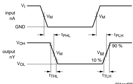
Measurement points are given in [Table 9](#).**Fig 5. Propagation delay data input (nA) to data output (nY) and transition time output (nY)****Table 9. Measurement points**
