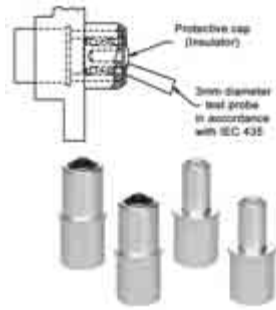
3 mm Diameter Test Probe in Accordance with IEC 435 Protective Cap (insulator)
