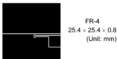
Fig. 5.1 Device Mounted on a Glass-Epoxy Board (a)
