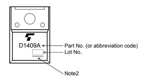
Note2: A line under a Lot No. identifies the indication of product Labels. Not underlined: [[Pb]]/INCLUDES > MCV Underlined: [[G]]/RoHS COMPATIBLE or [[G]]/RoHS [[Pb]]
