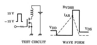
$$\begin{aligned} R_G &= 25~\Omega \\ V_{DD} &= 25~V,~L = 398~\mu H \end{aligned} \qquad EAS &= \frac{1}{2} \cdot L \cdot I^2 \cdot \left( \frac{BVDSS}{BVDSS - VDD} \right) \end{aligned}$$
