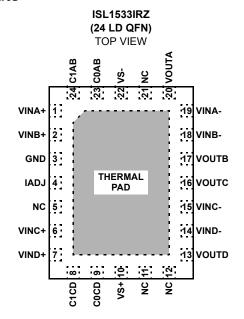
THERMAL PAD TO BE CONNECTED TO GND
