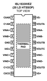
THERMAL PAD TO BE CONNECTED TO GND
