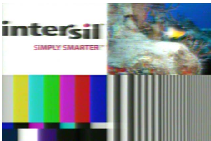
FIGURE 9. TEST PATTERN IMAGE AFTER 3000 FEET OF UNCOMPENSATED CAT 5
