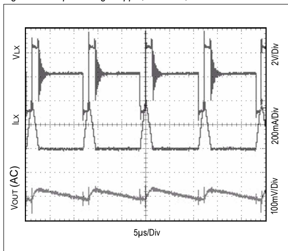
Figure 8. Output Voltage Ripple; V_{IN} = 2V , R_{load} = 100\Omega
