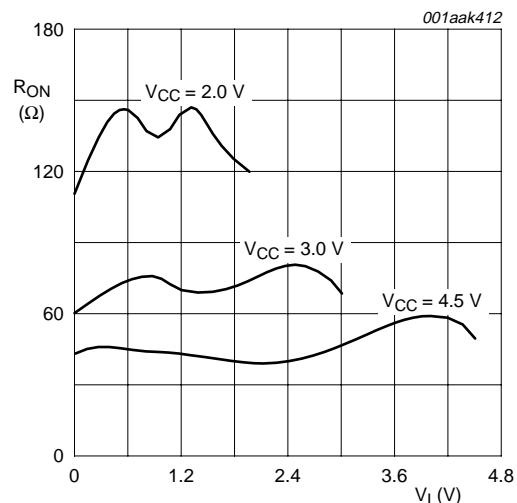
$V_i = 0 \text{ V to } V_{CC} - V_{EE}$
