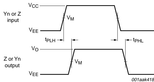
**Fig 13. Propagation delay input (An) to output (Yn)**
