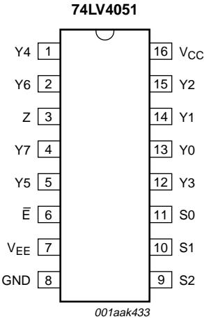
Fig. 5. Pin configuration SOT38-4 and SOT109-1
