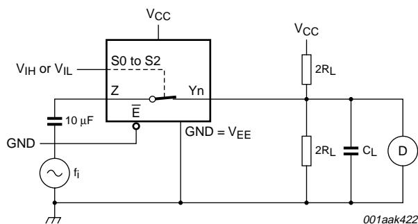
**Fig 20. Test circuit for measuring total harmonic distortion**
