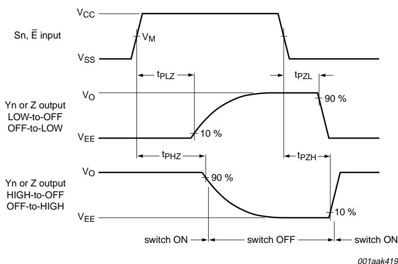
**Fig 14. Enable and disable times**
