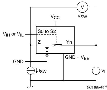
$$R_{ON} = V_{SW} / I_{SW}$$
