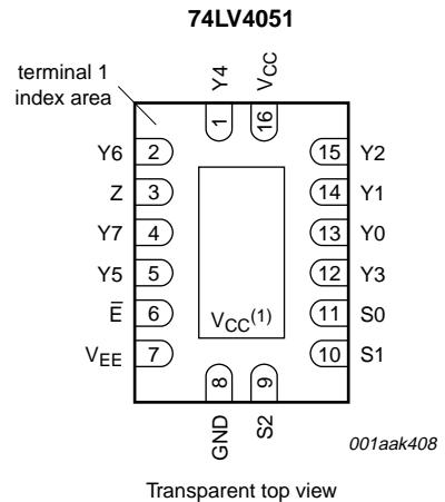
Fig. 7. Pin configuration for SOT763-1
