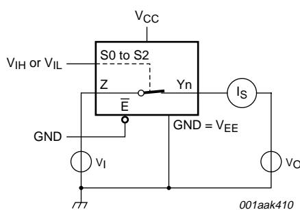
$V_I = V_{CC}$  or  $V_{EE}$  and  $V_O = \text{open circuit}$ .
