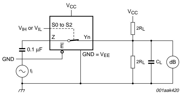
**Fig 16.** Test circuit for measuring frequency response
