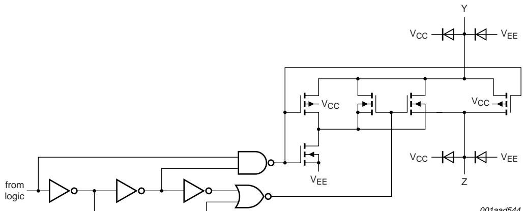
Fig 4. Schematic diagram (one switch)
