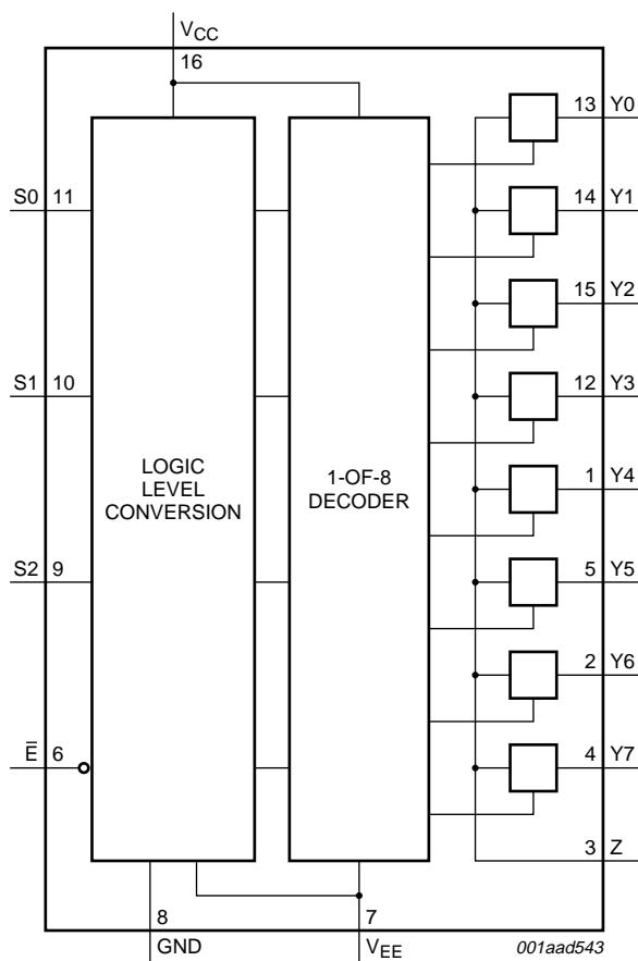
**Fig 1. Functional diagram**
