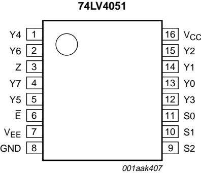
Fig. 6. Pin configuration SOT338-1 and SOT403-1
