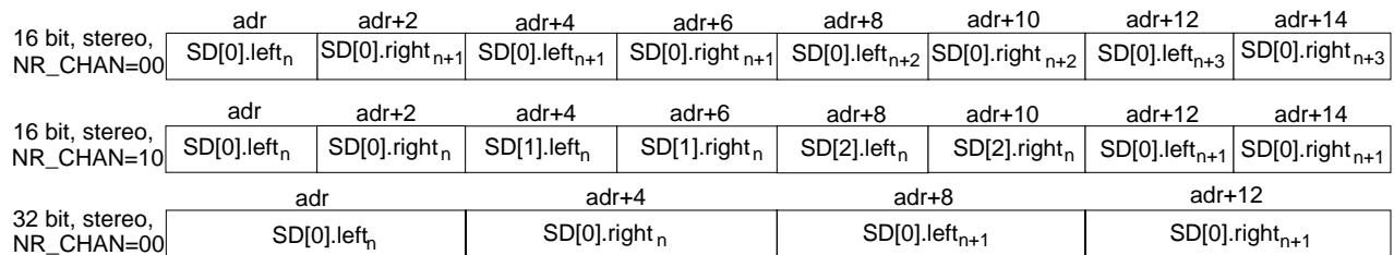
Figure 2: Examples of Audio Out Memory DMA Formats
