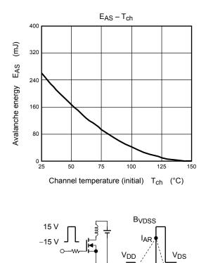
$$\begin{array}{ll} \mbox{Test circuit} & \mbox{Waveform} \\ \mbox{R}_G = 25 \ \Omega \\ \mbox{V}_{DD} = 90 \ \mbox{V}, \ \mbox{L} = 5.6 \ \mbox{mH} \end{array} \qquad E_{AS} = \frac{1}{2} \cdot \mbox{L} \cdot \mbox{I}^2 \cdot \left( \frac{\mbox{BVDSS}}{\mbox{BVDSS} - \mbox{V}_{DD}} \right) \end{array}$$
