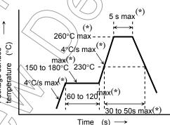
• The products are evaluated using above reflow soldering conditions. No additional test is performed exceed the condition (i.e. the condition more than (\*)MAX values) as a evaluation. Please perform reflow soldering under the above conditions.
