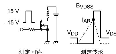
$$R_G = 25 \Omega, V_{DD} = 50 \text{ V} \quad E_{AS} = \frac{1}{2} \cdot L \cdot I^2 AR \cdot \left( \frac{B_{VDSS}}{B_{VDSS} - V_{DD}} \right)$$
