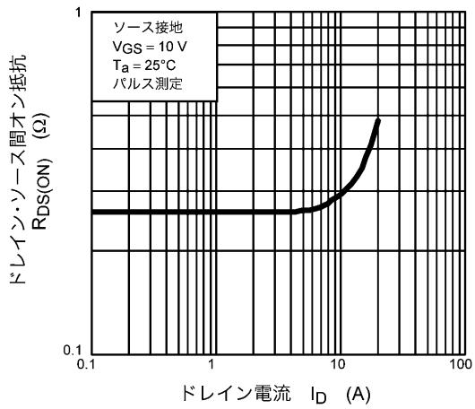
図 8.6  $R_{DS(\text{ON})}$  -  $I_D$
