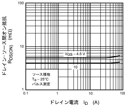
図 8.5  $R_{DS(\text{ON})} - I_D$
