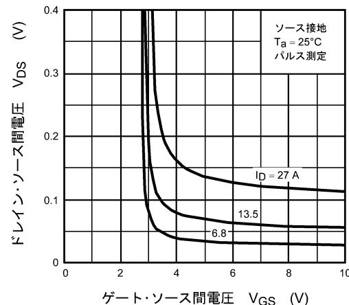
図 8.4  $V_{DS} - V_{GS}$
