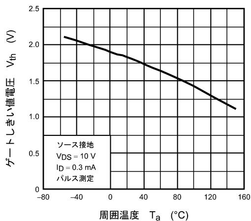
図 8.9  $V_{th}$  -  $T_a$
