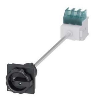
SENTRON, Switch disconnector 3LD, main switch, 3-pole, Iu: 25 A, Operating power / at AC-23 A at 400 V: 9.5 kW, floor mounting with door coupling, rotary operating mechanism, black, 4-hole mounting of the handle
