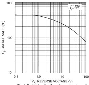
Fig. 4 Typical Junction Capacitance (per element)
