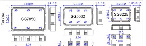
0.64 OE pin = HIGH : Specified frequency output OE pin = LOW: Output is high impedance #3 is connected to the cover.
