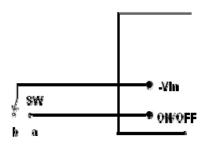
The converter output can be disabled by moving SW to position "a" – connected to –Vin with voltage level between -0.7 and 0.4V.
