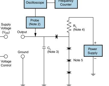
Note 1: An external  $0.1\mu F$  low frequency tantalum bypass capacitor in parallel with a  $0.01\mu F$  high frequency ceramic bypass capacitor close to the package ground and  $V_{DD}$  pin is required.
