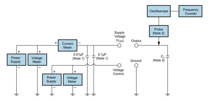
Note 1: An external  $0.1\mu F$  low frequency tantalum bypass capacitor in parallel with a  $0.01\mu F$  high frequency ceramic bypass capacitor close to the package ground and  $V_{DD}$  pin is required.
