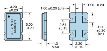
Note: Pin 1 Chamfer not shown.
