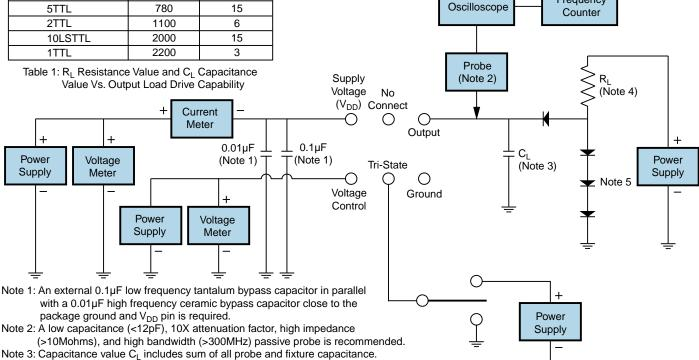
Note 4: Resistance value R<sub>1</sub> is shown in Table 1. See applicable specification sheet for
