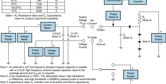
Note 4: Resistance value R<sub>1</sub> is shown in Table 1. See applicable specification sheet for 'Load Drive Capability'.
