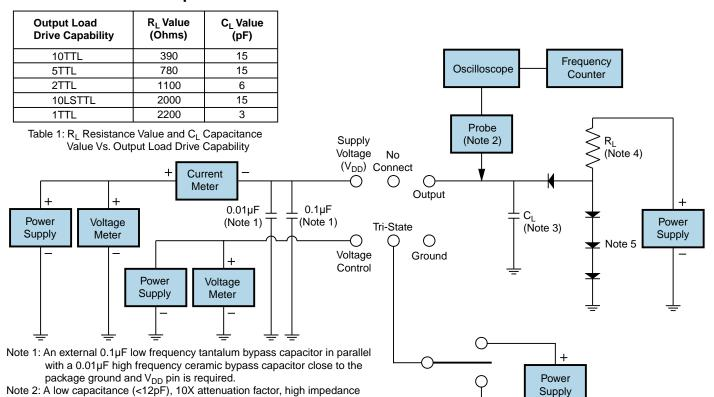
(>10Mohms), and high bandwidth (>300MHz) passive probe is recommended. Note 3: Capacitance value  $C_{\text{L}}$  includes sum of all probe and fixture capacitance.
