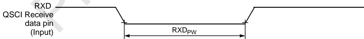
Figure 10-12 RXD Pulse Width
