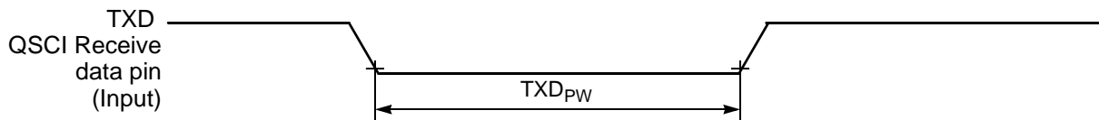
Figure 10-13 TXD Pulse Width
