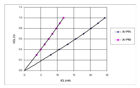
Figure 16-5. Typical 3-Volt Output Low Voltage versus Output Low Current (25°C)
