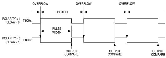
Figure 14-3. PWM Period and Pulse Width
