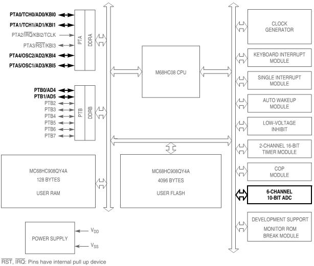
All port pins have programmable pull up device PTA[0:5]: Higher current sink and source capability PTB[0:7]: Not available on 8-pin devices
