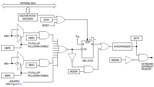
Figure 9-2. Keyboard Interrupt Block Diagram
