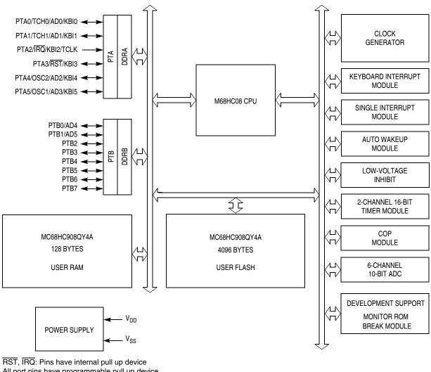
RST, IRQ: Pins have internal pull up device All port pins have programmable pull up device PTA[0:5]: Higher current sink and source capability PTB[0:7]: Not available on 8-pin devices
