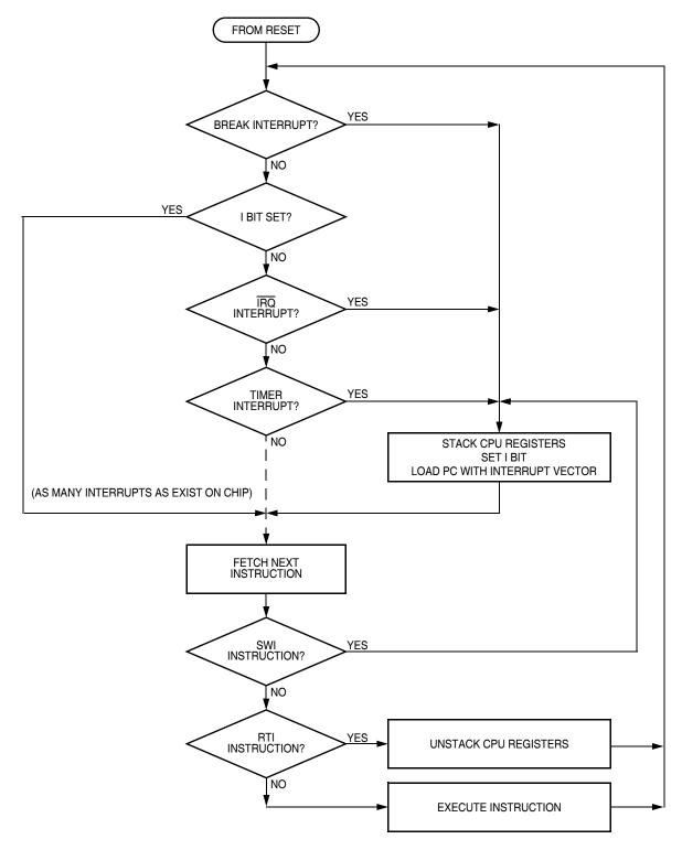
Figure 13-7. Interrupt Processing
