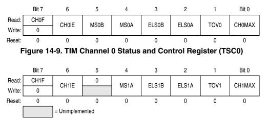
Figure 14-10. TIM Channel 1 Status and Control Register (TSC1)
