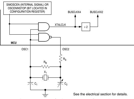
Figure 11-2. XTAL Oscillator External Connections
