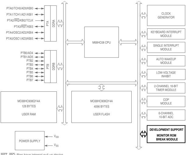
RST, IRQ: Pins have internal pull up device All port pins have programmable pull up device PTA[0:5]: Higher current sink and source capability PTB[0:7]: Not available on 8-pin devices
