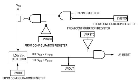
Figure 10-1. LVI Module Block Diagram
