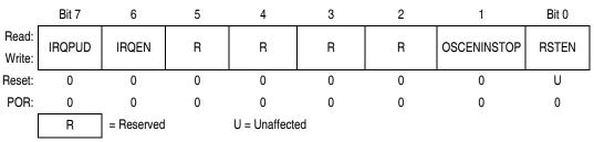
Figure 5-1. Configuration Register 2 (CONFIG2)
