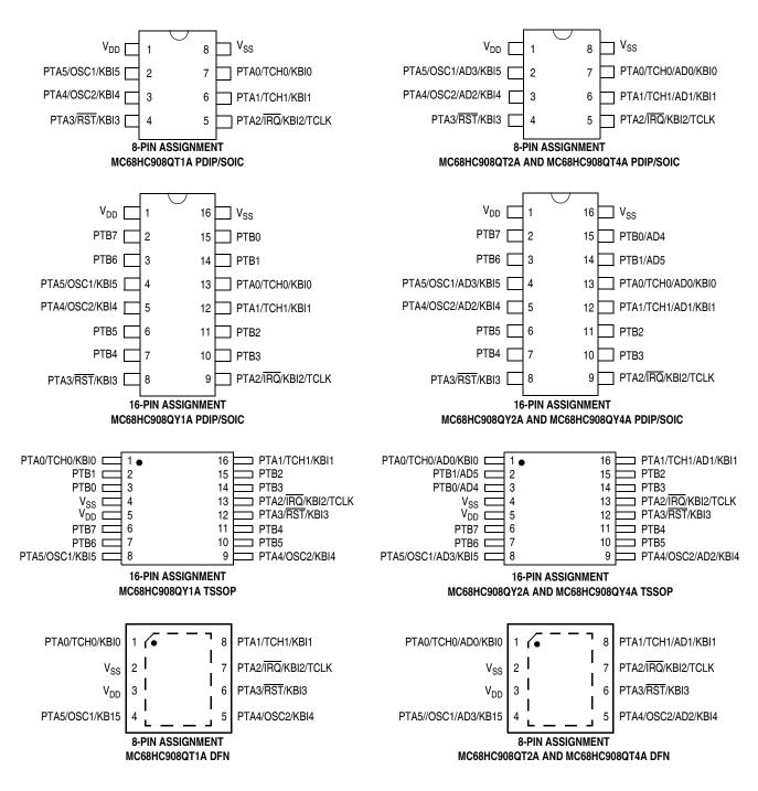
Figure 1-2. MCU Pin Assignments
