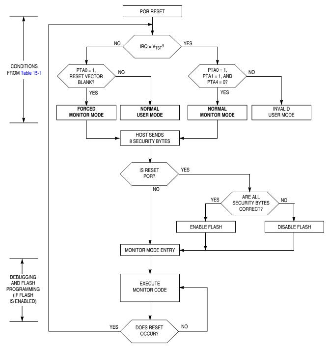
Figure 15-9. Simplified Monitor Mode Entry Flowchart
