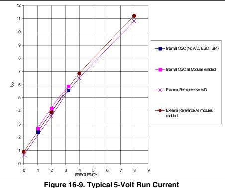
gure 16-9. Typical 5-Volt Run Curren versus Bus Frequency (25°C)
