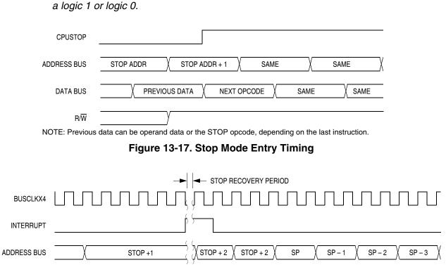
Figure 13-18. Stop Mode Recovery from Interrupt
