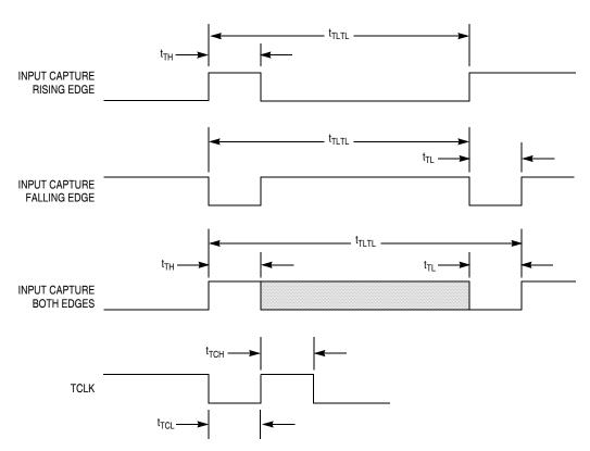
Figure 16-11. Timer Input Timing
