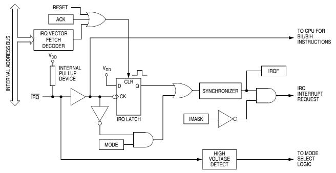
Figure 8-2. IRQ Module Block Diagram
