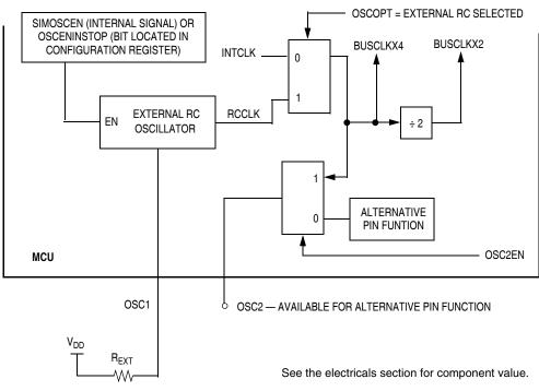
Figure 11-3. RC Oscillator External Connections
