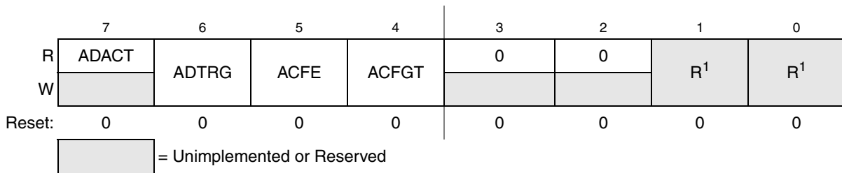
Figure 9-5. Status and Control Register 2 (ADCSC2)
