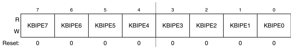
Figure 12-4. KBI Pin Enable Register
