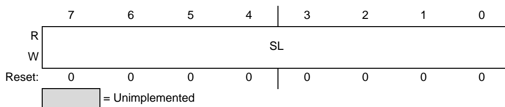
Figure 28. Sensitivity Threshold Register Format
