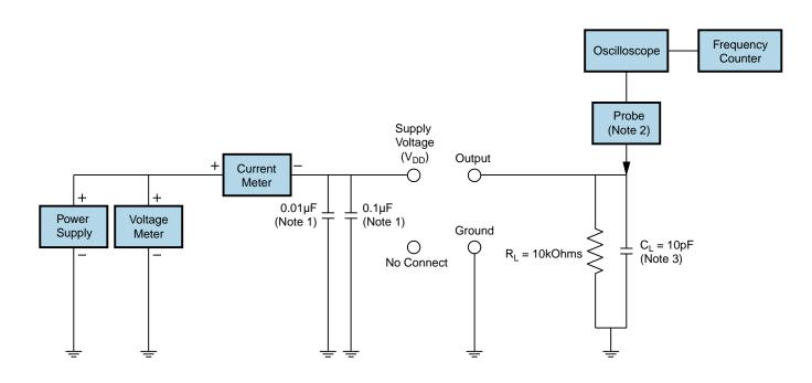
Note 1: An external 0.1µF low frequency tantalum bypass capacitor in parallel with a 0.01µF high frequency ceramic bypass capacitor close to the package ground and V<sub>DD</sub> pin is required.
