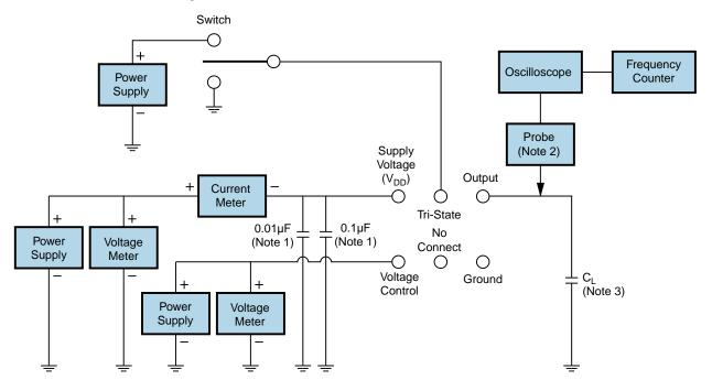
Note 1: An external  $0.1\mu F$  low frequency tantalum bypass capacitor in parallel with a  $0.01\mu F$  high frequency ceramic bypass capacitor close to the package ground and  $V_{DD}$  pin is required.
