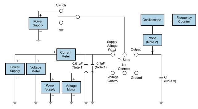
Note 1: An external  $0.1\mu$ F low frequency tantalum bypass capacitor in parallel with a  $0.01\mu$ F high frequency ceramic bypass capacitor close to the package ground and V<sub>DD</sub> pin is required.
