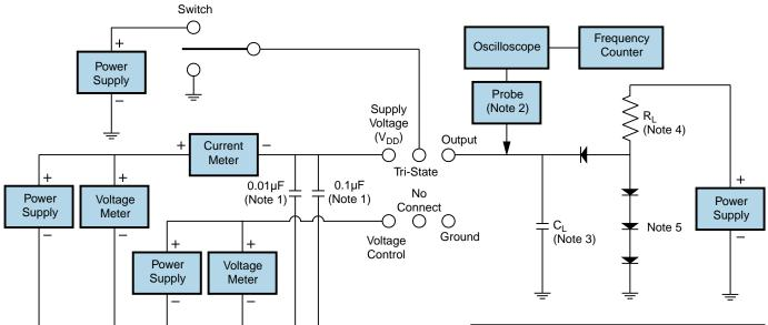
Note 1: An external  $0.1\mu F$  low frequency tantalum bypass capacitor in parallel with a  $0.01\mu F$  high frequency ceramic bypass capacitor close to the package ground and  $V_{DD}$  pin is required.
