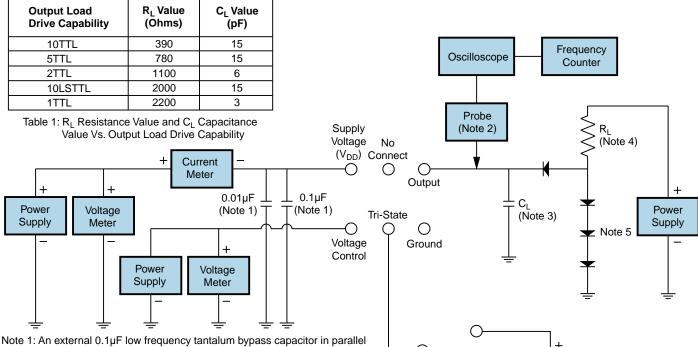
with a 0.01µF high frequency ceramic bypass capacitor close to the package ground and V<sub>DD</sub> pin is required.
