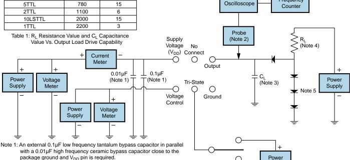
package ground and V<sub>DD</sub> pin is required. Note 2: A low capacitance (<12pF), 10X attenuation factor, high impedance (>10Mohms), and high bandwidth (>300MHz) passive probe is recommended.
