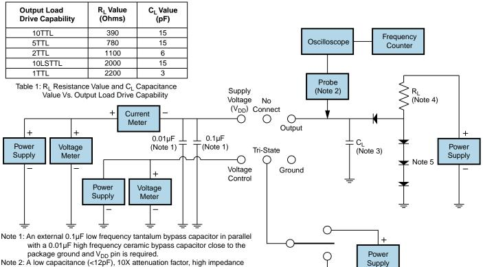
(>10Mohms), and high bandwidth (>300MHz) passive probe is recommended.
