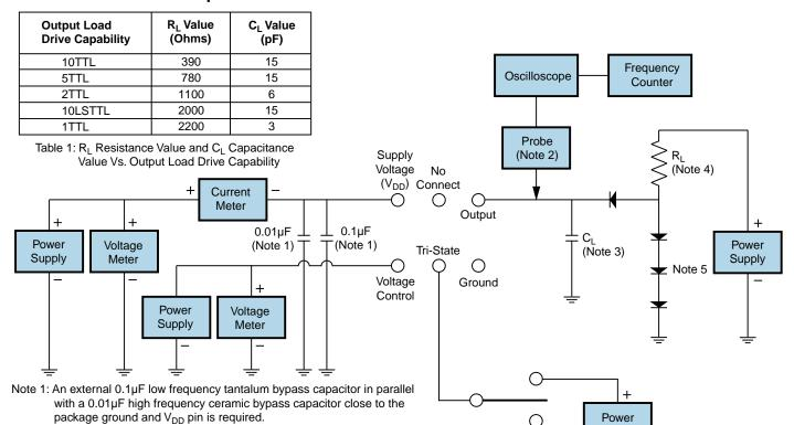
Note 2: A low capacitance (<12pF), 10X attenuation factor, high impedance (>10Mohms), and high bandwidth (>300MHz) passive probe is recommended.
