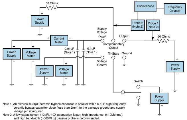
Note 3: Test circuit PCB traces need to be designed for a characteristic line impedance of 50 ohms.
