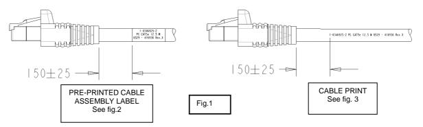
**REMARK** For cable assemblies <300mm the label or print will be placed in the middle of the cable.
